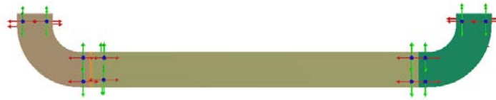
Figure 28: Clamping of end bar
